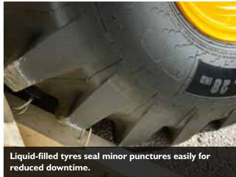
Liquid-filled tyres seal minor punctures easily for reduced downtime.
